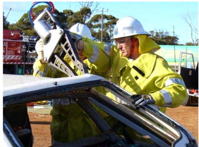
Reid Stubberfield and Derek Stanton using the jaws of life to cut through the roof of the car.
